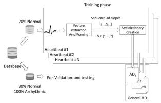
Fig. 2. Process to create a general antidictionary from a single record
