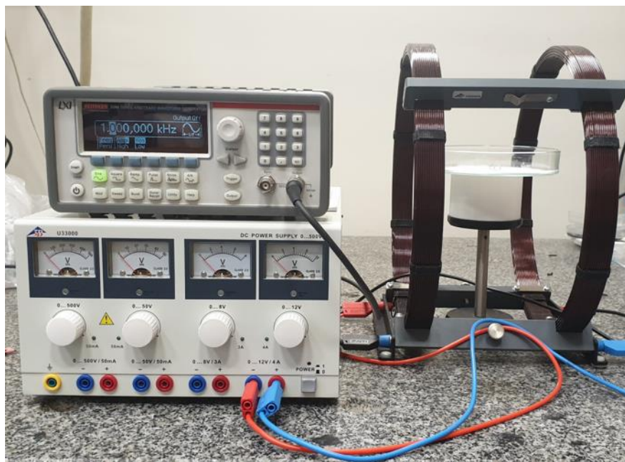
Figure S5: Experimental setup composed by Helmholtz coils used to test the magnetic devices.
