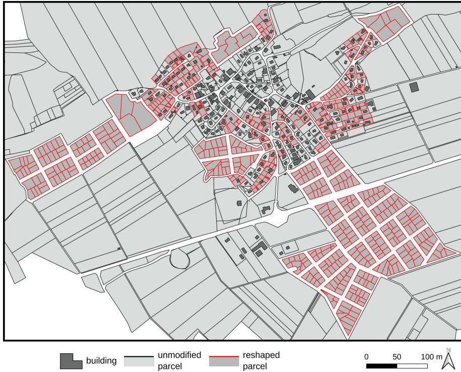
Figure 20: Simulation of the test scenario on the community of Gennes with the OBB-SS algorithm. Workflows Zone Division in the AU1 zones and Zone Consolidation in the AU2 zones. The width of peripheral roads has been set to 7 m. and the minimum width of contact between roads and parcels has been set to 12 m.
