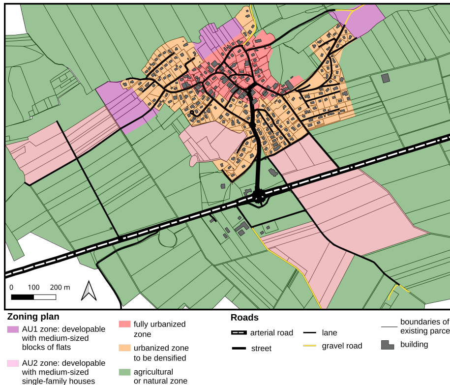
Figure 10: Zoning plan and parcel layout of the community of Gennes, east of France.
