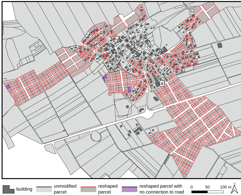
Figure 11: Simulation of the test scenario on the community of Gennes with the Oriented Bounding Box algorithm. Workflows Zone Division in the AU1 zones and Zone Consolidation in the AU2 zones.
