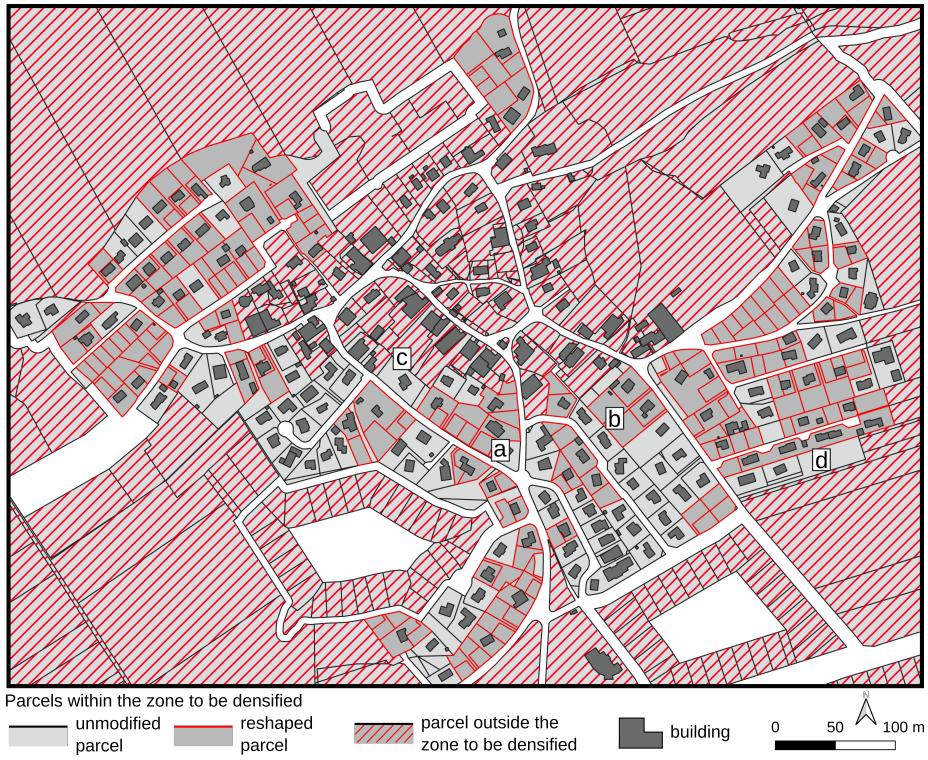
Figure 18: Simulation results obtained with the Parcel Densification workflow; small-sized houses planned to be built. Focus on the centre of the community of Gennes.
