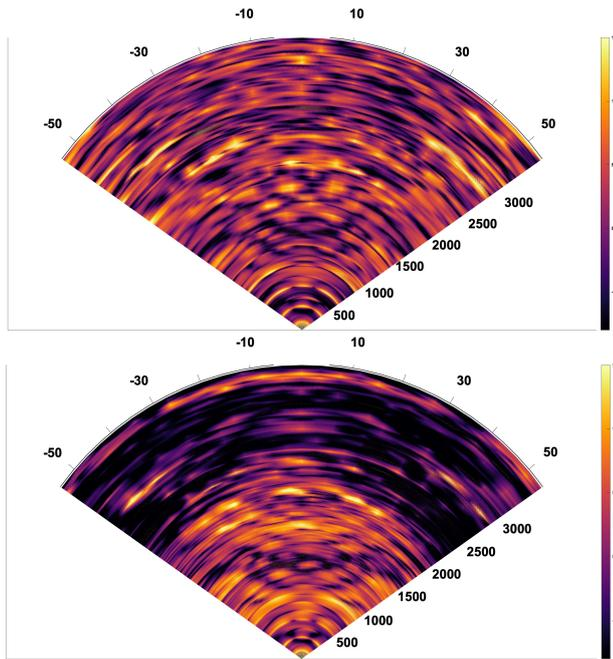
FIGURE 6 – Radiation spectra of measured facade (upper) and full dense cylinder matrix (lower). Data shown (spanning 23 dB) are normalised by the free-field propagation reference pressure of the same setup in absence of any elements of the scattering system.
