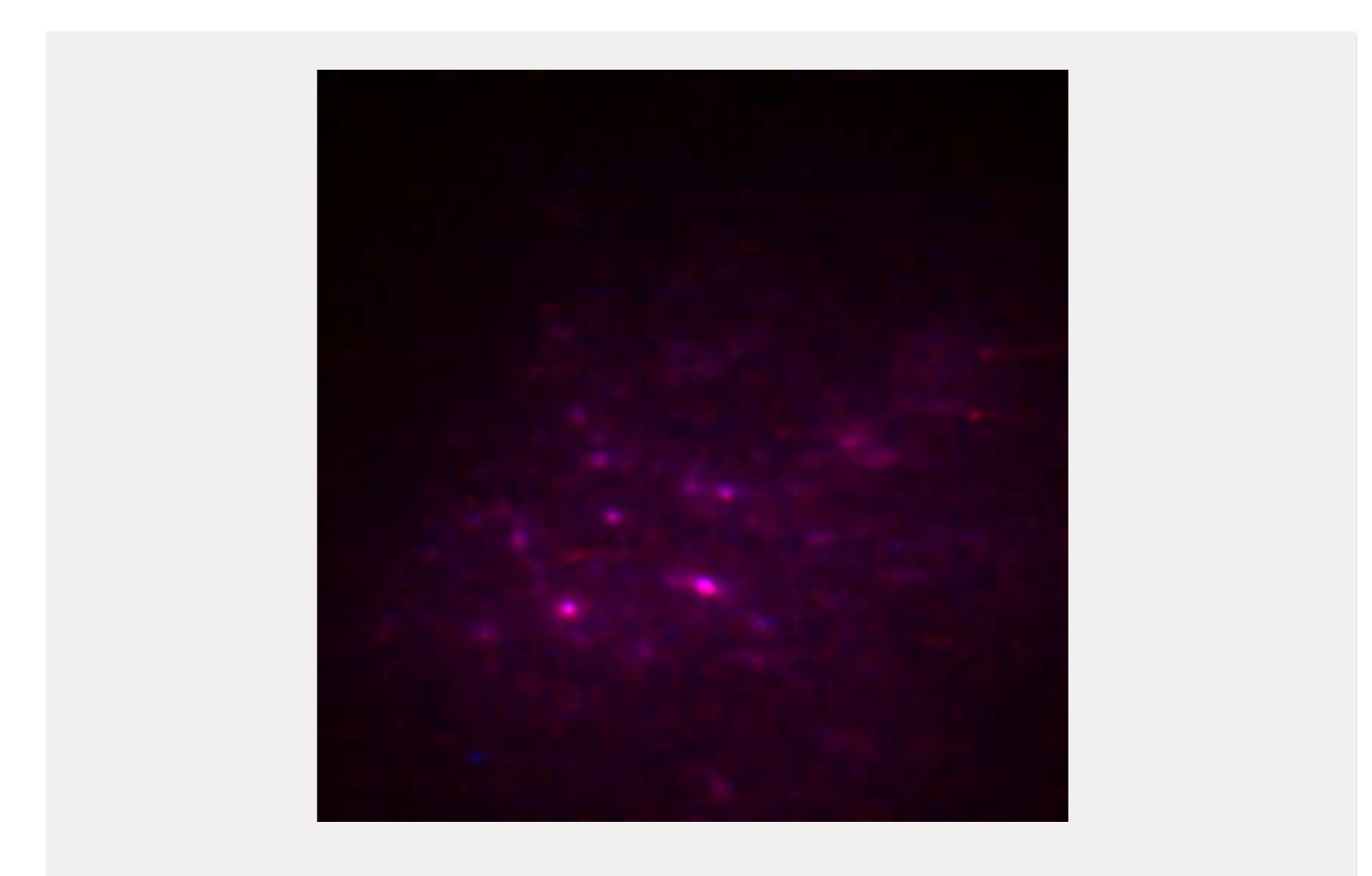
Image composed from the images obtained in IR-OSL (red channel) and in BL-OSL (blue channel); Fluvial sediment (Somme river, Epagne-Epagnette) irradiated at 300 Gy - ©CAD A. Zink
