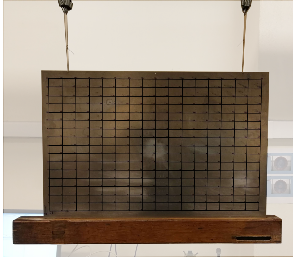
Figure 13: Structure under test - Clamped plate suspended to a rigid frame by bungee cords
