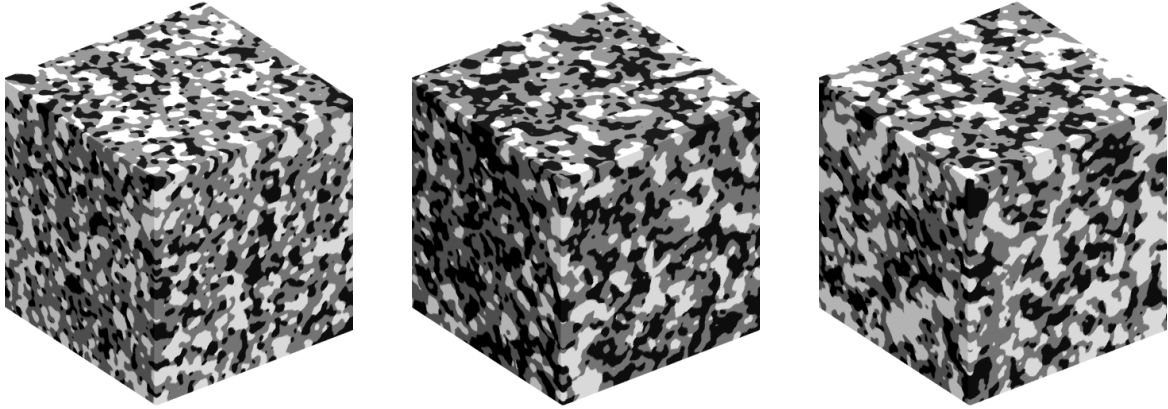
Figure 1. 3D reconstruction of three real microstructures. Cubes of 12.5 \mu\text{m} side ( 250^3 voxels). From left to right, the operating time of the cell is 0 h, 1500 h and 2000 h. The porous, YSZ and Ni phase are respectively black, gray and white.
