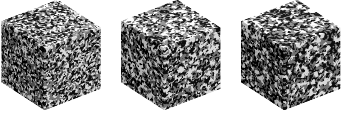
Figure 3. 3D rendering volume of three synthetic microstructures. Cubes of 17.5 \mu\text{m} side ( 350^3 voxels). From left to right, the parameters \lambda_p = \lambda_{YSZ} = 2.10^{-3} , \theta = 3 and \sigma = 5 are constants, whereas \lambda_{Ni} \in \{2.10^{-3}; 1.10^{-4}; 5.10^{-5}\} and \lambda_c \in \{1; 20; 40\} . The porous, YSZ and Ni phase are respectively black, gray and white.
