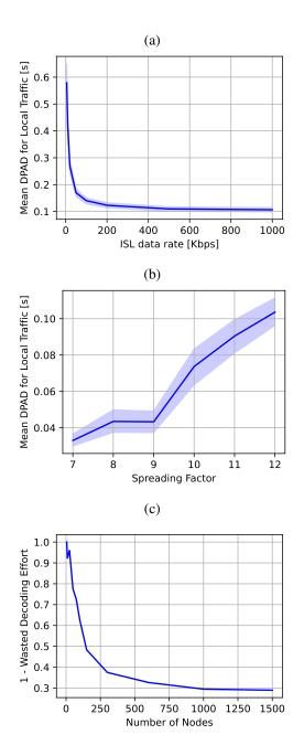
Fig. 6. Mean DPAD for local traffic for varying ISL data rate (a) and for varying SF (b). The Effective Decoding effort ratio (1 - Wasted Decoding Effort) is shown in (c) (shadowed area indicates 95% CI)
