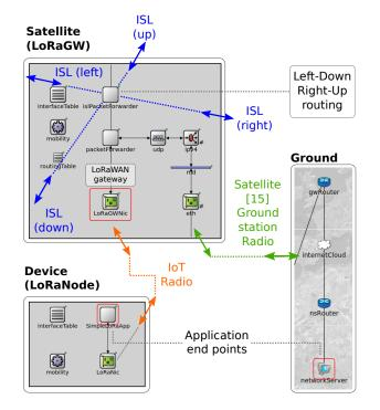
Fig. 3. FLORASAT architecture: terrestrial device, satellite, and ground segments.
