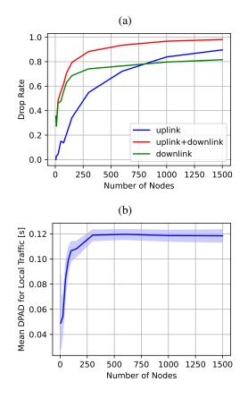
Fig. 5. Drop Rate due to collisions (a) and mean DPAD for frames destined to the local node (b) (shadowed area indicates 95% CI)
