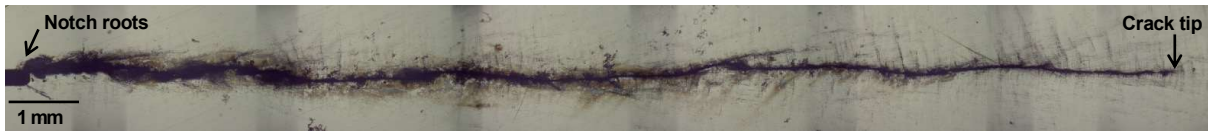
Figure 7: Optical observation of nearly transverse secondary branches in mode II for 16NCD13 steel (test #2)
