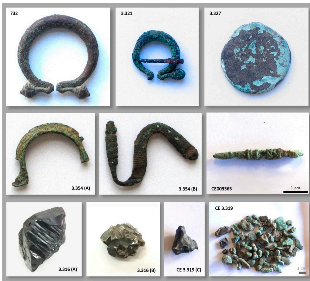
Figure 6. Examples of some of the artefacts analyzed by pXRF from Outeiro de Baltar hillfort at the Museo Arqueológico Provincial de Ourense (Galicia, Spain), which include fibulae (732; 3.321; 3.354 (A); 3.354 (B)), a coin (3.327), a decorated pin (CE003363), a cassiterite crystal (3.316 (A)), pyrite crystals (3.316 (B)), a tin slag (CE 3.319 (C)) and metal scrap nodules (CE 3.319). Black scale applies to all artefacts' photographs, and gray scale (bottom right) only applies to the CE 3.319 photograph.
