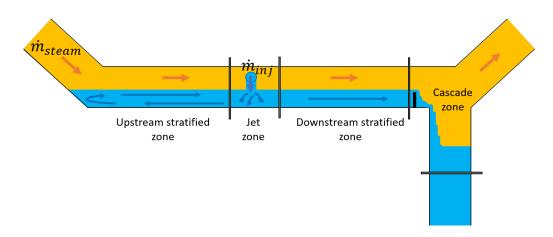
Fig. 5 Phenomenology in the COSI test section.
