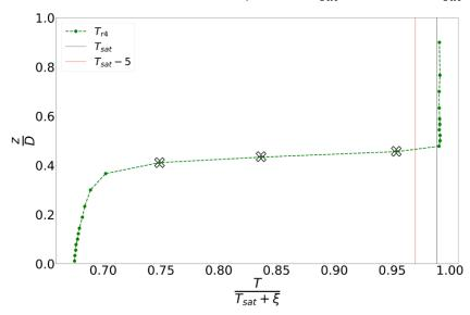
Fig. 15 Typical time-averaged temperature profile of a rake in a TOPFLOW-PTS test.
