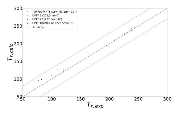
**Fig. 25** Prediction of the mean liquid temperature against the validation database. In Table 10, the indicators in Eqn. (5) are computed.
