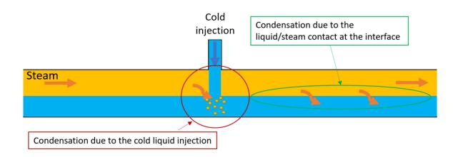
Fig. 1 Main phenomena occurring at a sub-cooled injection into a two-phase flow.
