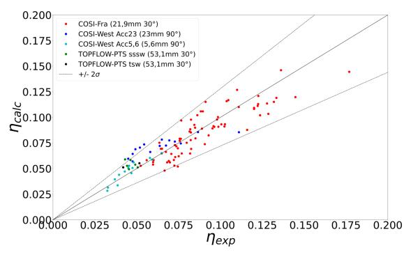
Fig. 23 Fitting of the new condensation correlation over the assessment database.
