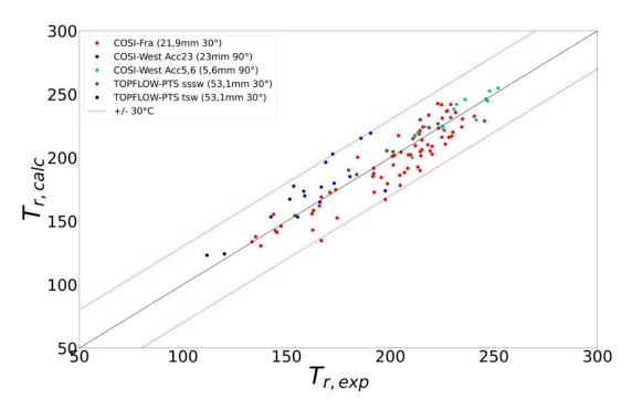
Fig. 24 Prediction of the mean liquid temperature against the assessment database.
