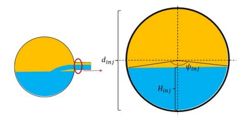
Fig. 12 Stratified flow in the UPTF injection pipe.
