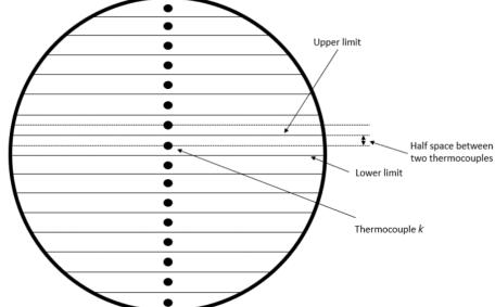
Fig. 16 Thermocouple associated surfaces estimation for a COSI rake.
