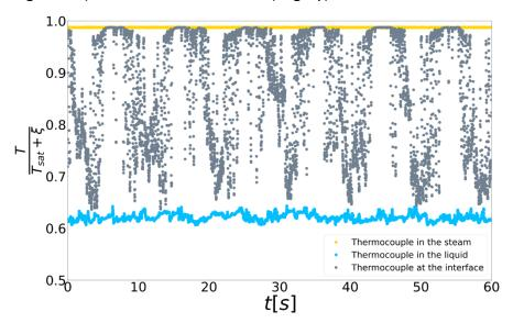
**Fig. 14** Typical temperature profiles in time in a TOPFLOW-PTS test.
