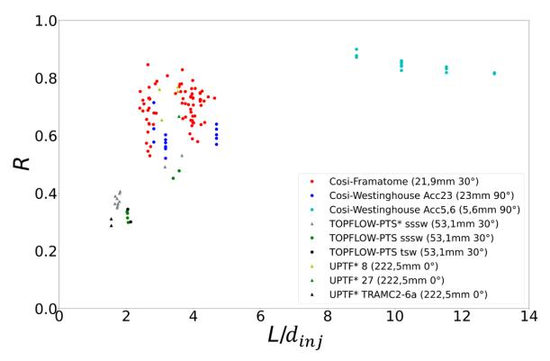
**Fig. 22** Condensation potential R plotted against the jet length over diameter ratio. The triangles are the validation tests (also marked as \* in the legend).
