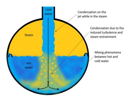
Fig. 2 Main local DCC phenomena occurring at the injection.
