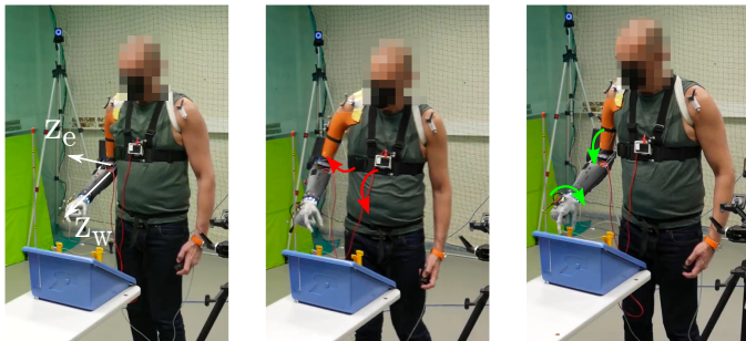
(a) The prosthesis user wants to pick the clothespin, which requires simultaneous wrist pronation (around z_w ) and elbow extension. (around z_e ). (b) With an initially still prosthesis, the user starts mobilizing task-oriented upper arm and torso compensations (in red). (c) Compensations are detected and used to generate adequate prosthesis motions (in green), which naturally leads the user to cancel compensatory motions.
