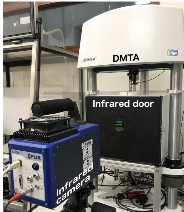
Figure 1: Thermography setup in front of the DMTA
