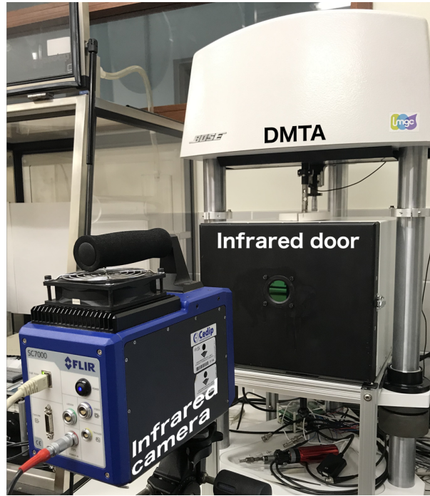
Figure 1: Thermography setup in front of the DMTA (BOSE ELF 3230)
