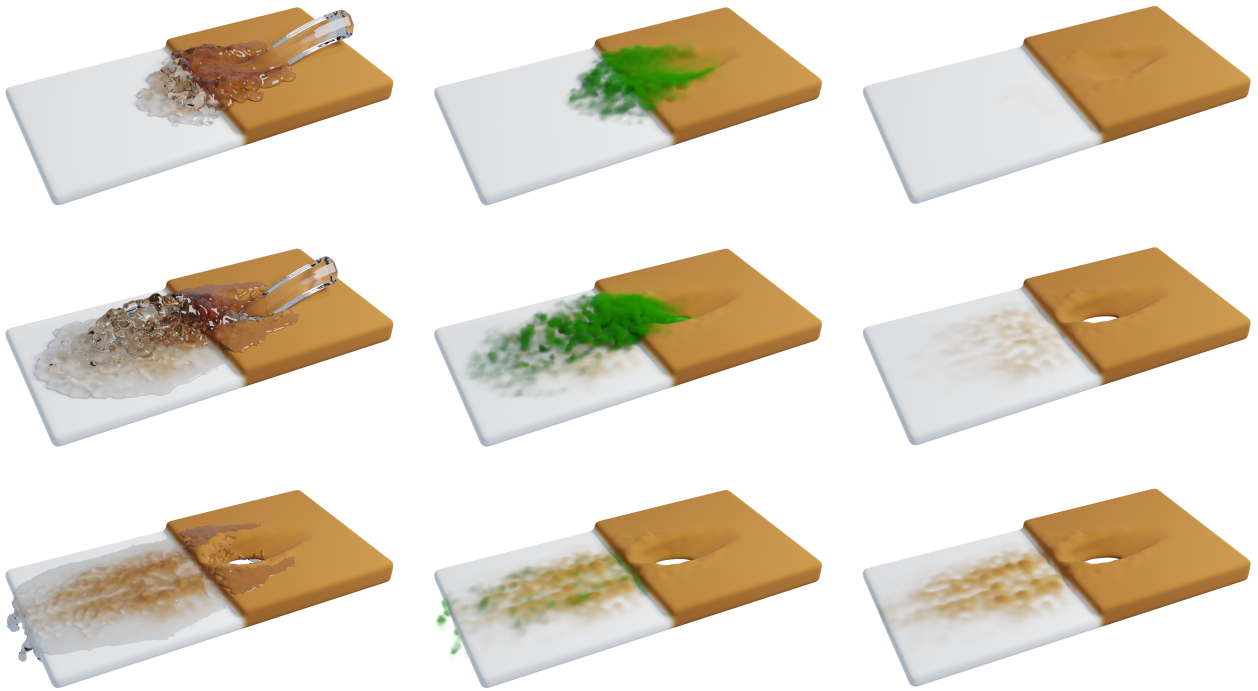
2 Figure 5 depicts the erosion, sediment transport and sediment deposition of a brittle material over an immutable 3 one. The solid phase is composed of 28000 particles and interacts with 6000 fluid particles. The transfer rate 4 between solid materials and sediments is controlled by \kappa_{\text{erosion}} (set to 5 \cdot 10^{-3} ). We choose a sediment radius 5 r^{s_k} = 0.1 to model dirt or sand with no diffusivity (i.e. D^{s_k} = 0 ).
