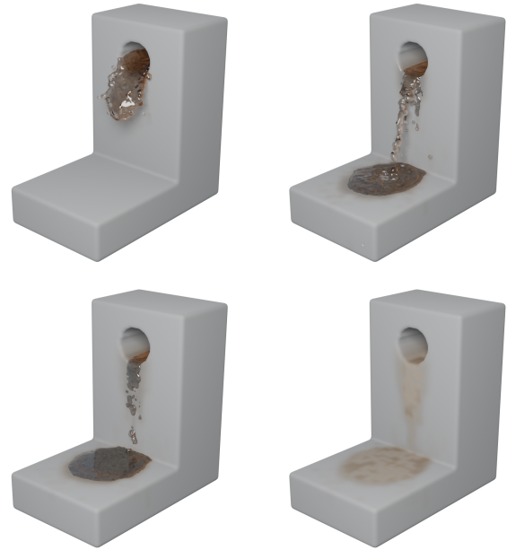
Figure 8: Stains produced by dirty water coming out of a hole. It shows diffusion of water and sediments in the medium and deposition on the surface after evaporation.
