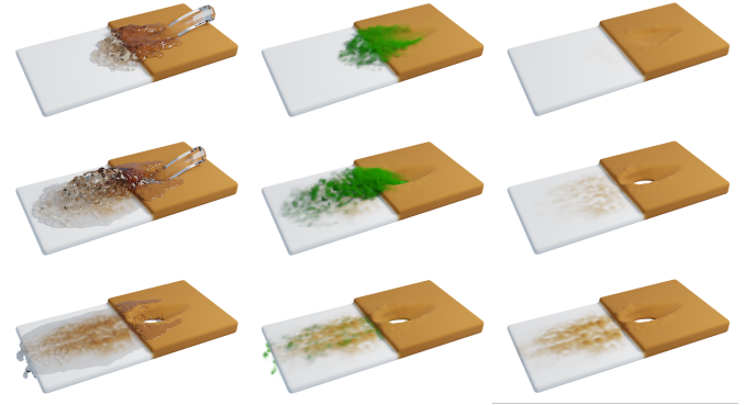
Figure 5: Erosion, transport and deposition of a brittle material (brown) over an immutable material (white). Each row depicts a specific simulation step. From left to right: simulation result, sediments shown in green within the fluid, solid particles only.
