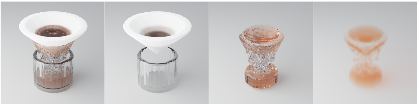
Figure 1: Coffee is dissolved in the water that gets inside the filter. Concentrated water then seeps through the filter to reach the glass. From left to right: Render of the scene, solid and wetting, fluid and its contained sediments, sediments density.
