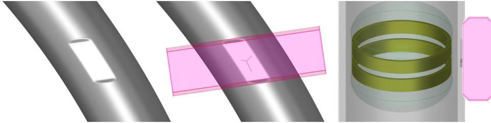
**Figure 15.** SG tube: testing configuration. An axial probe made of two coils used in differential mode (shown in right image) moves along the tube axis. The anti-vibration bar (see center image) induces wear on the tube surface (see left image). In addition, a surface-breaking crack may appear (shown on center and right images).
