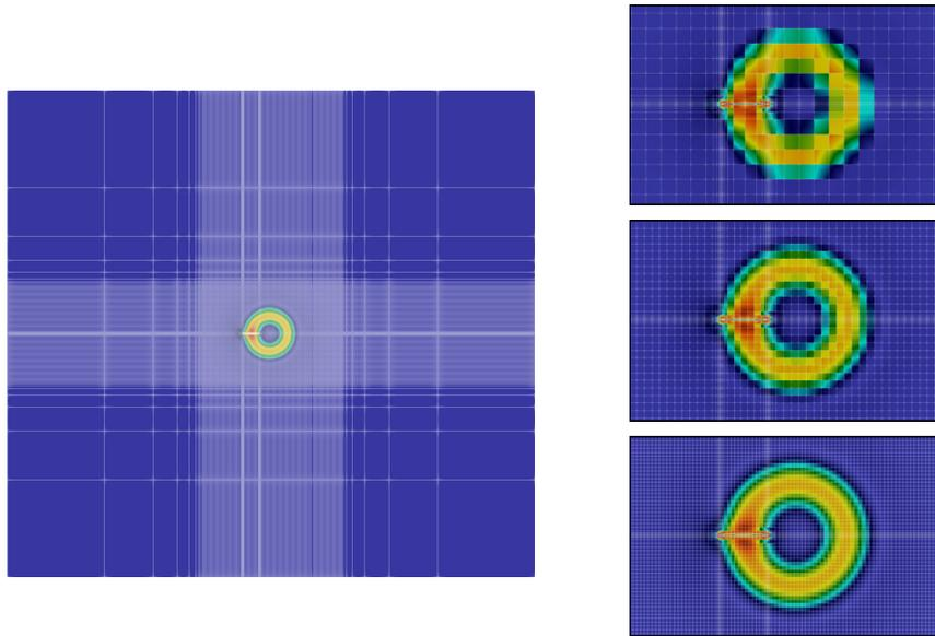
**Figure 13.** TEAM 15 benchmark: mesh 3 and surface current density  $\text{Im}(\mathbf{J}_s)$  for the coil at  $x = 13.75$  mm (left); close-ups of the slot region showing details of meshes 1 to 3 (right, top to bottom).
