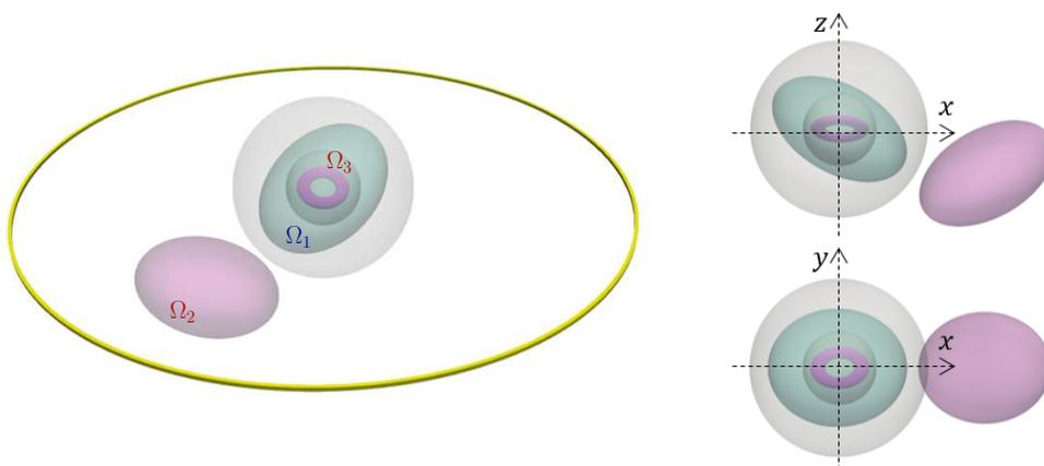
**Figure 8.** Multi-body example: sketch of the configuration showing the coil (left panel only), the nonconductive or reasonably conductive ellipsoidal body, the disjoint ellipsoidal conductive body, the internal toroidal conductive body, and the two spherical evaluation surfaces.
