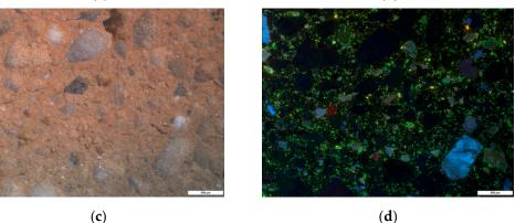
Figure 2. Observations in CL-imagery for ceramic fragments made by hand: sample BDX 24419 ((a) white light reflectance, (b) cathodoluminescence emission); and sample BDX 24420 ((c) white light reflectance, (d) cathodoluminescence emission).
