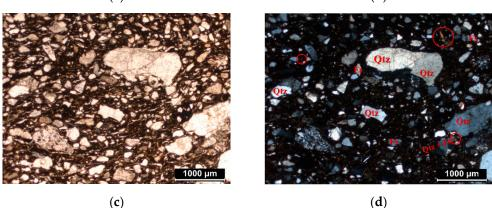
**Figure 1.** Petrographic observations: observation on matrix of BDX 24418 ((**a**) plane-polarized light, (**b**) cross-polarized light); observation of matrix of BDX 24419 ((**c**) plane-polarized light, (**d**) cross-polarized light). The identified minerals are mainly quartz (Qtz), altered feldspars (Fs) and mica (indicated by the circle).
