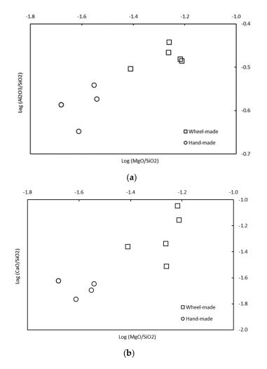
**Figure 4.** Binary diagrams of potsherds (square-shape potsherds made by hand; circle-shape potsherds made by wheel) expressed in log Al<sub>2</sub>O<sub>2</sub>/Si-log MgO/SiO<sub>2</sub> (**a**) and log CaO/SiO<sub>2</sub>-log MgO/SiO<sub>2</sub> (**b**). Hand-made samples BDX 24419 and BDX 24421 present very close values, so their points are overlapping.
