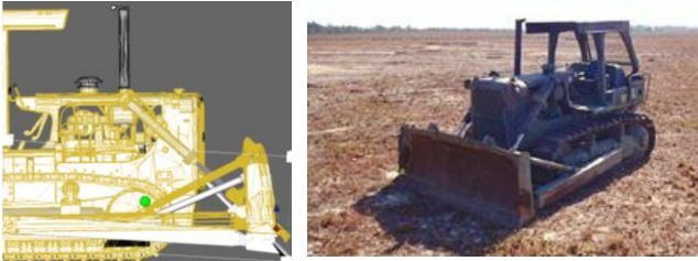
Figure 4. Comparison of our CAD (left) and ground truth (right). The actual blade position is represented in yellow, and the estimated ground truth is in white.
