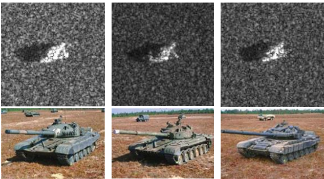
Figure 1 Comparison between SAR images (top) and photo (bottom) of the three MSTAR variants of the T72.
