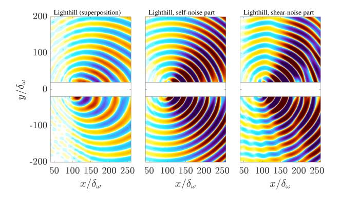
Fig. 7 Far-field radiation characteristics of the fluctuating pressure fields p', on the left the result of the Lighthill's equation (1) regarding the superposition of the self-noise and the shear-noise result, in the middle the results of the self-noise contribution, and on the right the result of shear-noise contribution. The source region in the middle of each plot is shaded white. The plots use a color scale minimum and maximum value of  $\pm 15$  Pa.
