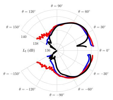
Fig. 8 Directivity of the acoustic intensity magnitude  $L_{\rm I}$  depending on the angle  $\theta$ , along a circle at the vortex pairing location  $x/\delta_{\omega}=110$  and  $x/\delta_{\omega}=0$  with a radius of  $r/\delta_{\omega}=140$ . The results inside the mixing layer are excluded due to the high values inside the source region. Legend: — DNS, — Lighthill's equation, — AWE-PO.
