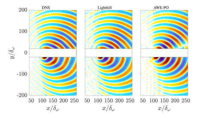
Fig. 6 Far-field radiation characteristics of the fluctuating pressure fields p', on the left the result of the DNS, in the middle the results of Lighthill's equation (1), and on the right the result of AWE-PO (5). The source region in the middle of each plot is shaded white. The plots use a color scale minimum and maximum value of  $\pm 15$  Pa.
