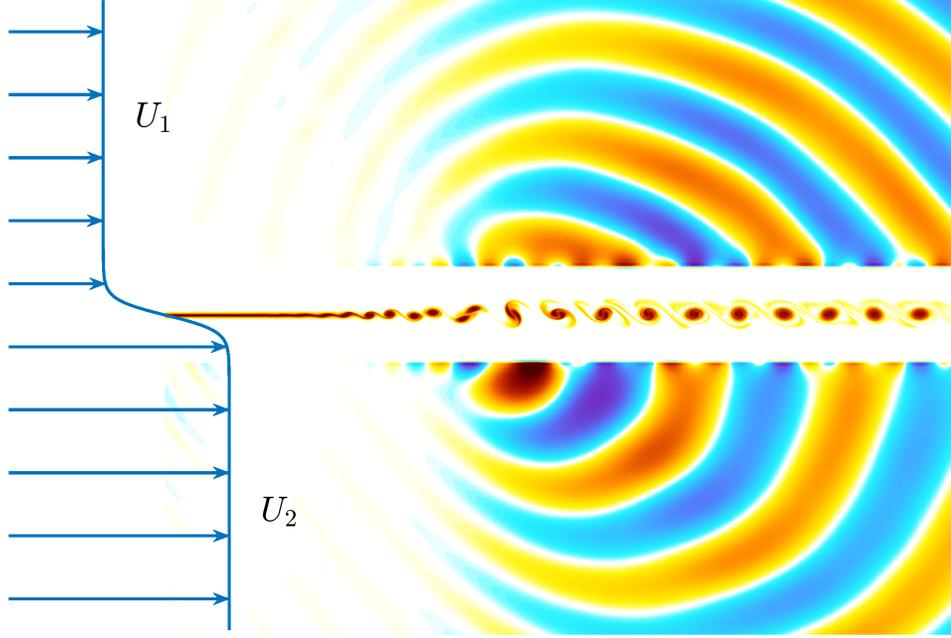
**Fig. 1** Schematic view of the mixing layer. Instantaneous vorticity and fluctuating pressure fields are represented at the center and periphery of the shear zone, respectively. Only a part of the domain is shown.
