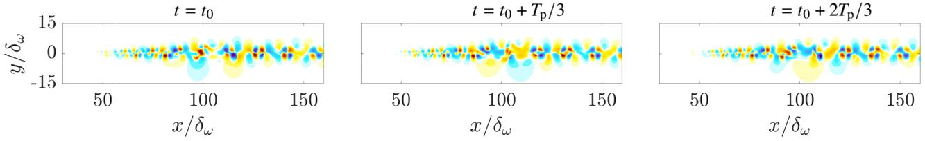
**Fig. 5 Visualization of the right-hand-side of AWE-PO (2), using a color scale minimum and maximum of  $\pm 3 \cdot 10^9 \text{ kg}/(\text{m}^3\text{s}^2)$ , respectively. Comparability to the other source plots is achieved by including a relevant pre-factor  $1/(c_0^2\Delta t)$  to obtain the solution variable  $p'$  after solving AWE-PO for the scalar potential  $\phi$ .**
