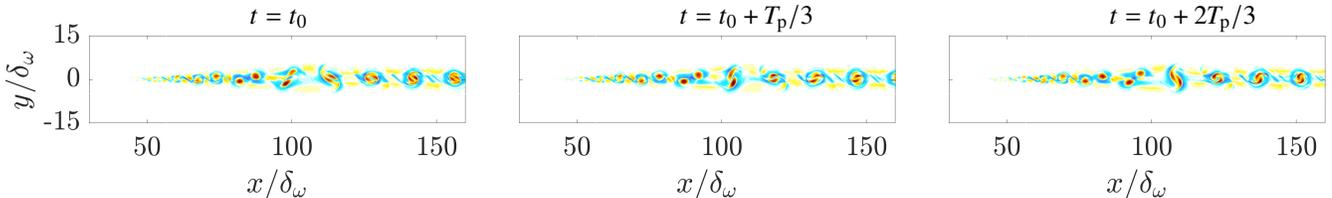
**Fig. 4** Self-noise part of Lighthill's right-hand-side term, which is the source of equation (3), using a color scale minimum and maximum of  $\pm 3 \cdot 10^{10} \text{ kg}/(\text{m}^3\text{s}^2)$ , respectively.
