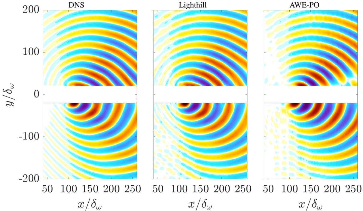
**Fig. 6** Far-field radiation characteristics of the fluctuating pressure fields  $p'$ , on the left the result of the DNS, in the middle the results of Lighthill's equation (1), and on the right the result of AWE-PO (5). The source region in the middle of each plot is shaded white. The plots use a color scale minimum and maximum value of  $\pm 15$  Pa.
