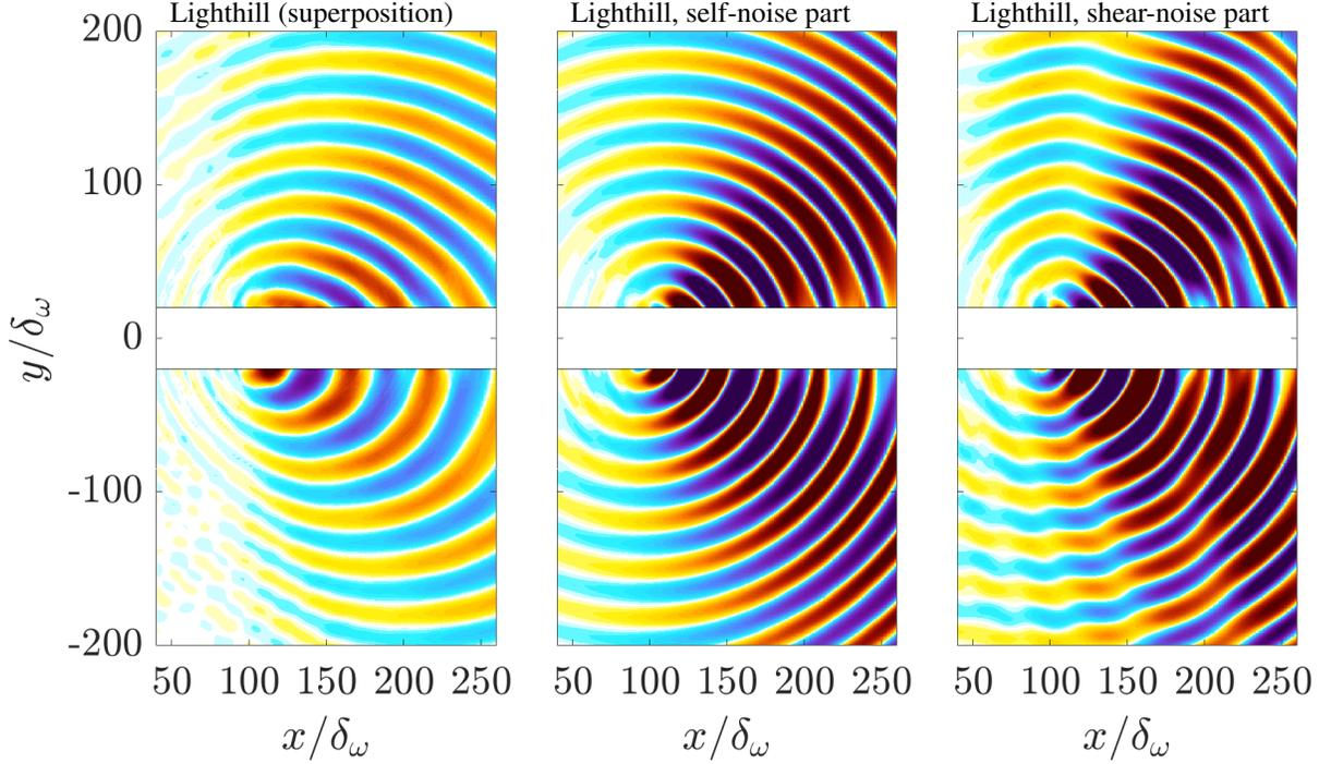
**Fig. 7** Far-field radiation characteristics of the fluctuating pressure fields  $p'$ , on the left the result of the Lighthill's equation (1) regarding the superposition of the self-noise and the shear-noise result, in the middle the results of the self-noise contribution, and on the right the result of shear-noise contribution. The source region in the middle of each plot is shaded white. The plots use a color scale minimum and maximum value of  $\pm 15$  Pa.
