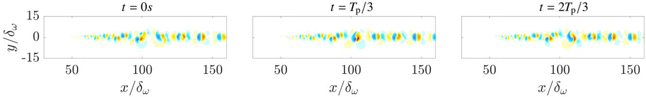
**Fig. 9** Visualization of the partial time derivative part of the right-hand-side of AWE-PO (2), using a color scale minimum and maximum of  $\pm 3 \cdot 10^{10} \text{ kg}/(\text{m}^3\text{s}^2)$ , respectively. Comparability to the other source plots is achieved by including a relevant pre-factor  $1/(c_0^2\Delta t)$  to obtain the solution variable  $p'$  after solving AWE-PO for the scalar potential  $\phi$ .
