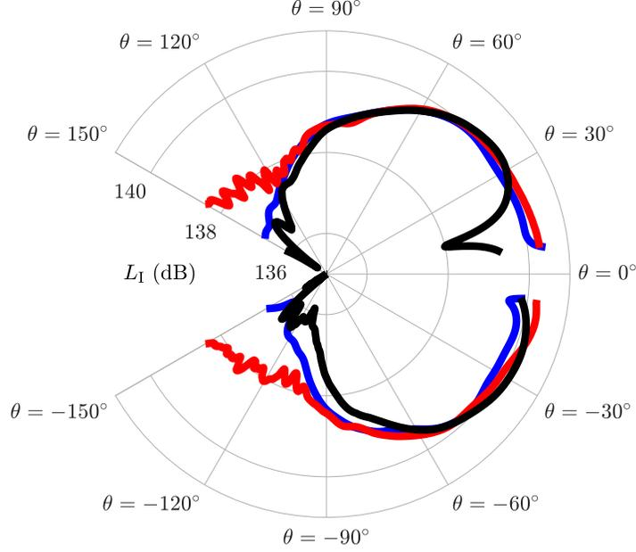
**Fig. 8** Directivity of the acoustic intensity magnitude  $L_I$  depending on the angle  $\theta$ , along a circle at the vortex pairing location  $x/\delta_\omega = 110$  and  $x/\delta_\omega = 0$  with a radius of  $r/\delta_\omega = 140$ . The results inside the mixing layer are excluded due to the high values inside the source region. Legend: — DNS, — Lighthill’s equation, — AWE-PO.
