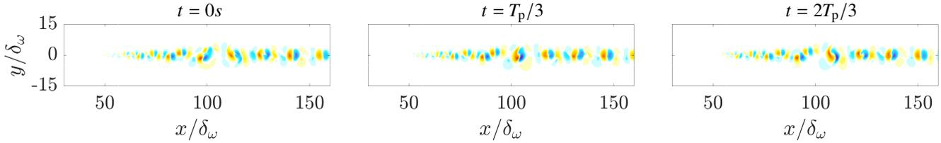
**Fig. 10** Visualization of the convective derivative part of the right-hand-side of AWE-PO (2), using a color scale minimum and maximum of  $\pm 3 \cdot 10^{10} \text{ kg}/(\text{m}^3\text{s}^2)$ , respectively. Comparability to the other source plots is achieved by including a relevant pre-factor  $1/(c_0^2\Delta t)$  to obtain the solution variable  $p'$  after solving AWE-PO for the scalar potential  $\phi$ .
