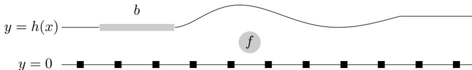
Figure 1: Parametrization of a slowly variable waveguide of width  $h$ . A wavefield  $u$  is generated by an internal source  $f$  and/or a boundary source  $b$ . Squares represent measurements of  $u$  taken on the surface  $y = 0$ .
