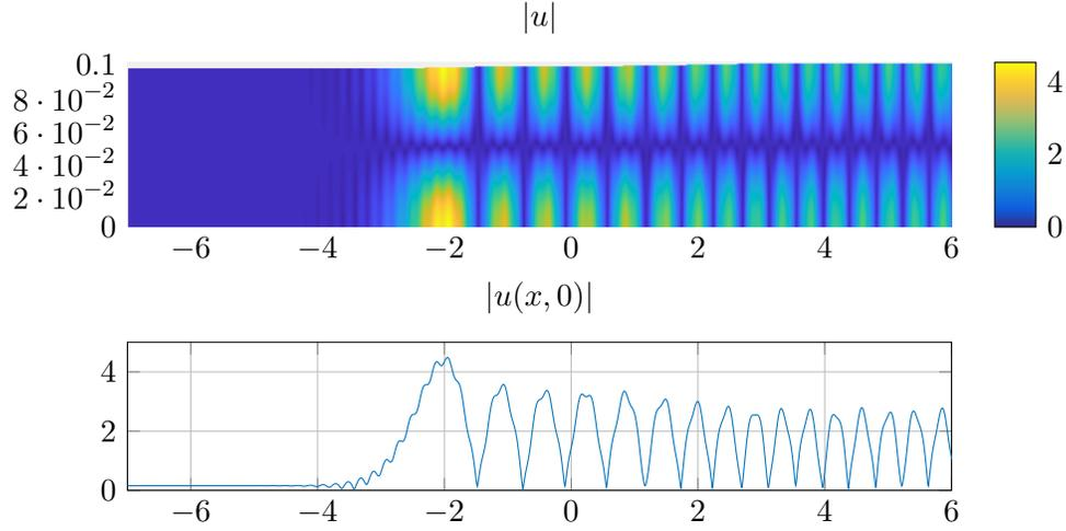
Figure 6: Illustration of the amplitude of the wavefield measurements in a varying waveguide. The wavefield  $u$  is solution of (7) where the profile  $h$  is given in (51) and  $k = 31.5$  is a locally resonant frequency. Data are generated using the finite element method described in Section 5.1. Top: amplitude of  $|u|$  in the whole waveguide  $\Omega$  (non scaled). Bottom: amplitude of the measurements of  $|u|$  on the surface  $y = 0$ .
