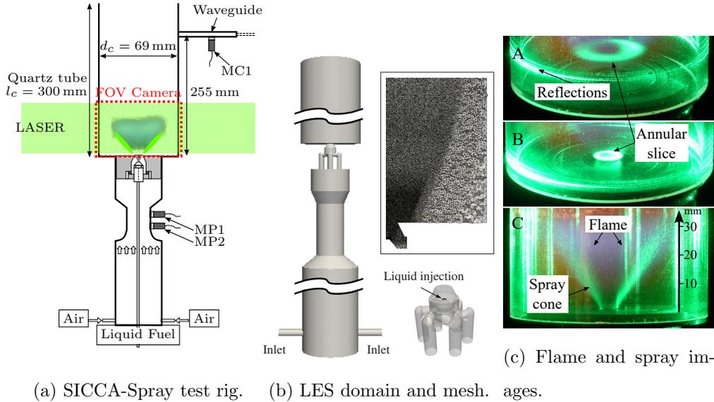
(a) SICCA-Spray test rig. (b) LES domain and mesh. (c) Flame and spray images.
