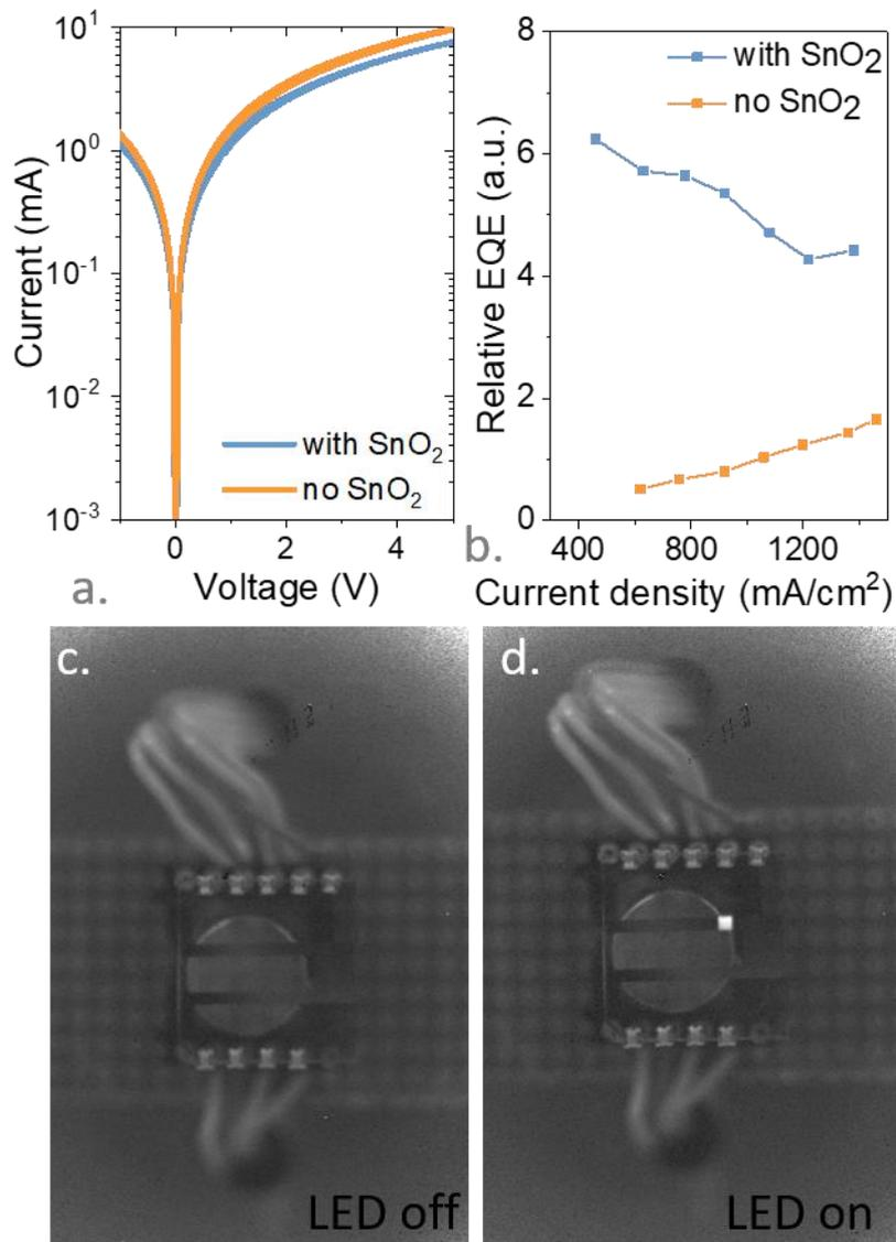
**Figure 6 Benefit of SnO<sub>2</sub> layer for electroluminescence.** a. IV curves of the LED stack with and without SnO<sub>2</sub> layer under forward bias. b. Relative EQE of the LED stack with and without SnO<sub>2</sub> layer under large forward bias. Image of the diode collected through a filter at 1.4  $\mu\text{m}$  on a InGaAs camera while the LED is off (c.) and on (d.). The diode is operated at room temperature under 5 mA in this case.
