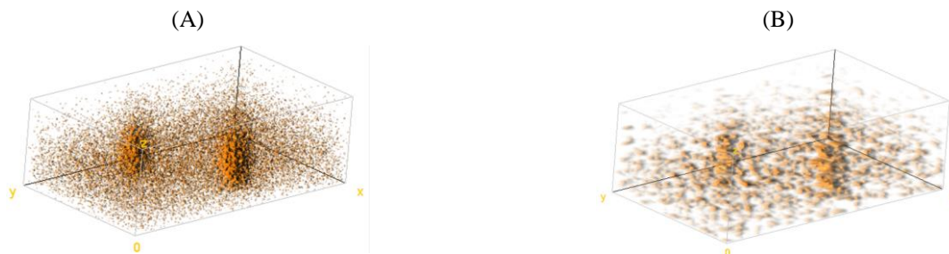
Figure 3. Scientific image of SARS-Cov-2 produced by our instrumental and computational pipeline FAMOUS. A. A 3D representation of the raw acquisitions of the free viral particles. B. The reconstructed representation of the raw acquisition, thanks to the computational strategy contained into FAMOUS.
