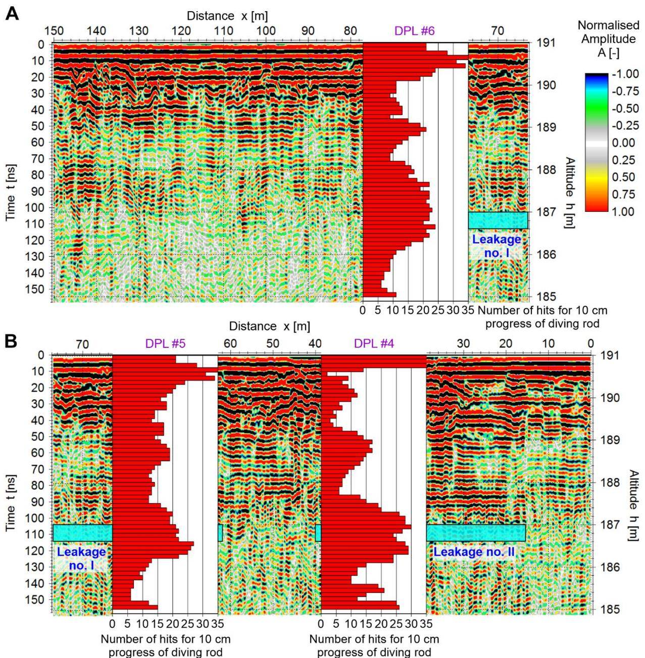
**Figure 9.** Superposition of information from Figure 8 for different antennae orientations: (A) profile section 70 ÷ 150 m; and (B) profile section 0 ÷ 70 m.
