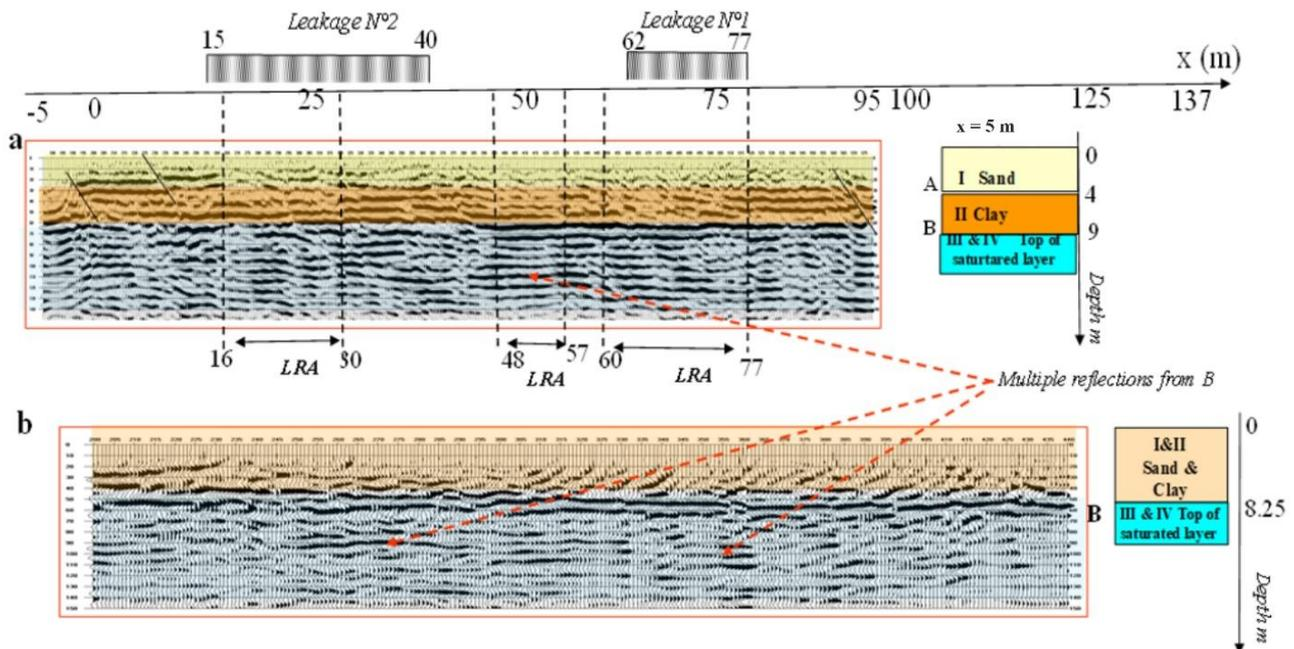
**Figure 12.** The high-resolution seismic reflection profiles obtained along the top of dike and their interpretation. (a) The 100 Hz profile, LRA symbols indicate the loss of reflection, straight black lines indicate shallow faults; (b) 26 Hz profile.
