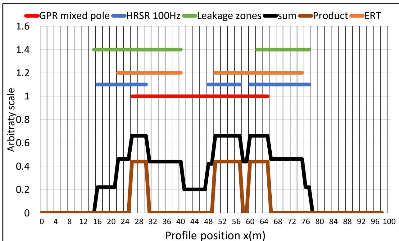
**Figure 13.** Symbolic illustration of detected hazard zones, detected by GPR, ERT, and HRSR, in profile intervals between 0 and 100 m. The “sum” and “product” denote, respectively, the scales fusion of three used methods by using the fuzzy logic: the logic “or” and logic “and”, respectively.
