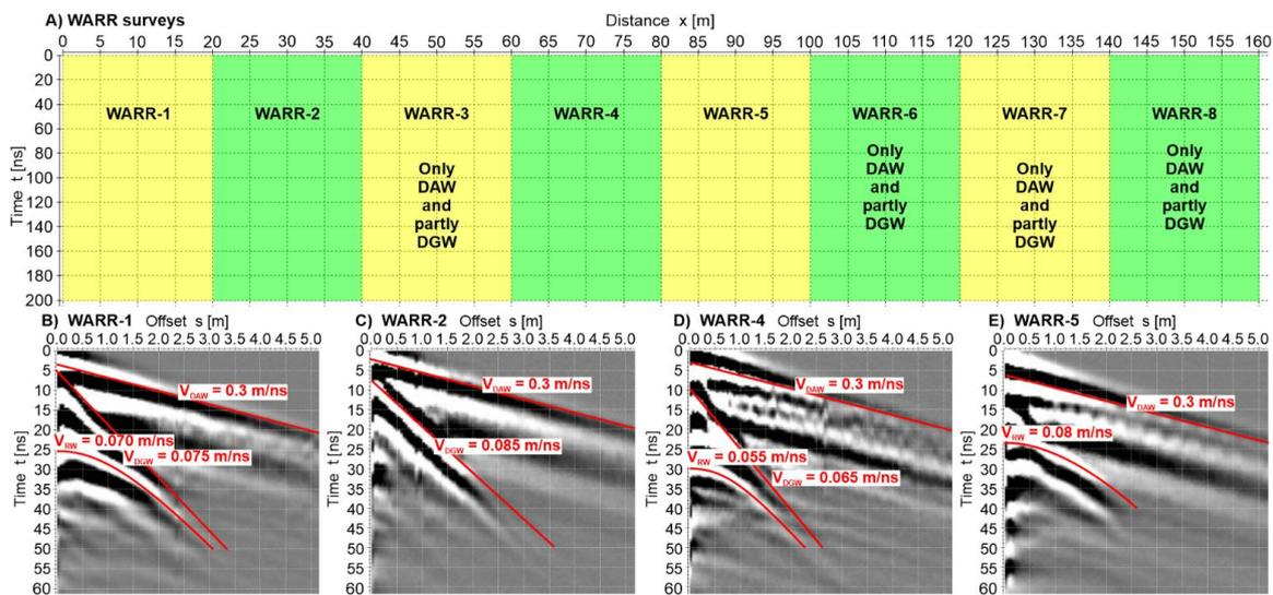
**Figure 4.** (A) Location of WARR surveys along profile GPR-2 (crown of dike); (B) First five meters of WARR Hodograph recorded from  $x = 0$  m to  $x = 20$  m; (C) First five meters of WARR Hodograph recorded from  $x = 20$  m to  $x = 40$  m; (D) First five meters of WARR Hodograph recorded from  $x = 60$  m to  $x = 80$  m; (E) First five meters of WARR Hodograph recorded from  $x = 80$  m to  $x = 100$  m.
