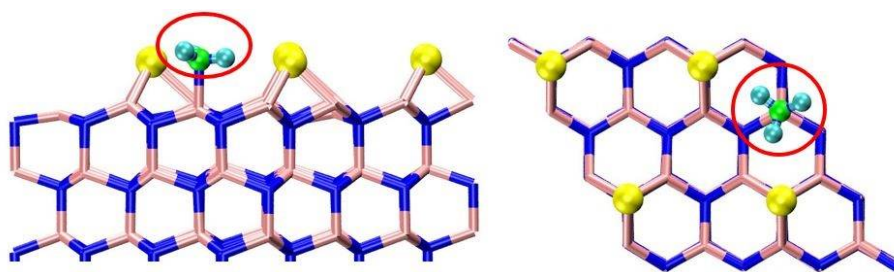
Fig. 3. Side and top views of the stable structure found in which the \text{NH}_3 is adsorbed on a \text{Ga(T1)} atom, highlighted inside the red circle. Details are provided in the text and the color code for the atoms is identical to the former figures.
