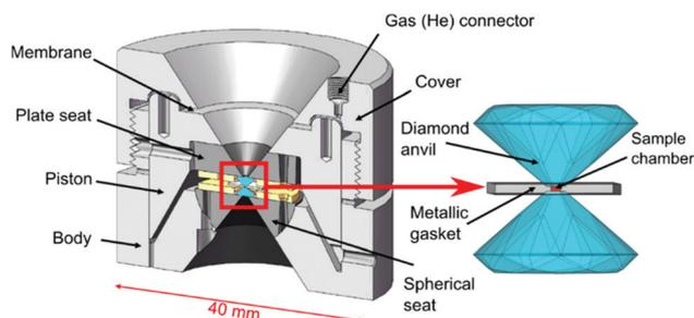
Fig. 22 Section view of a membrane diamond anvil cell.
