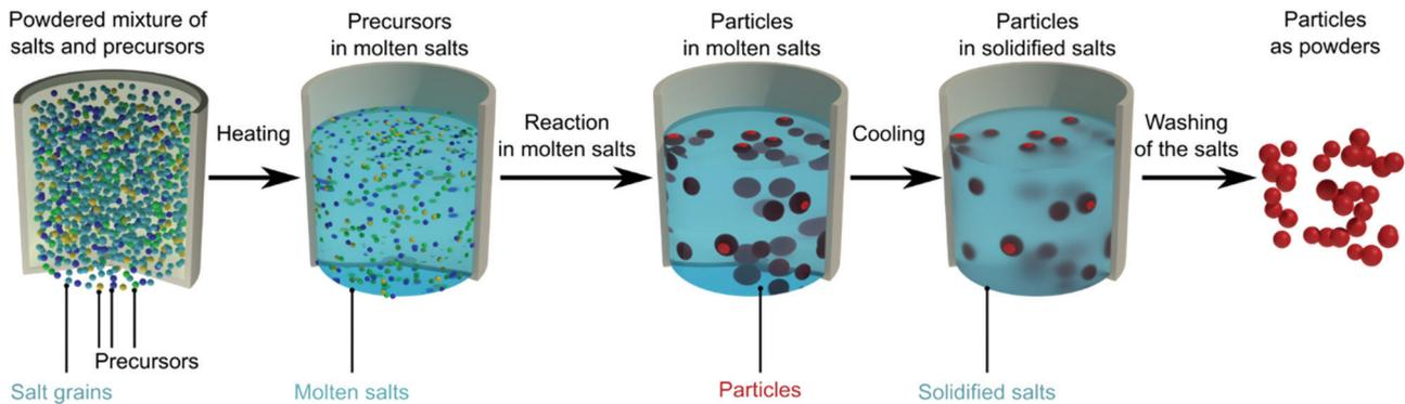
Fig. 16 Basic procedure for molten salt synthesis.
