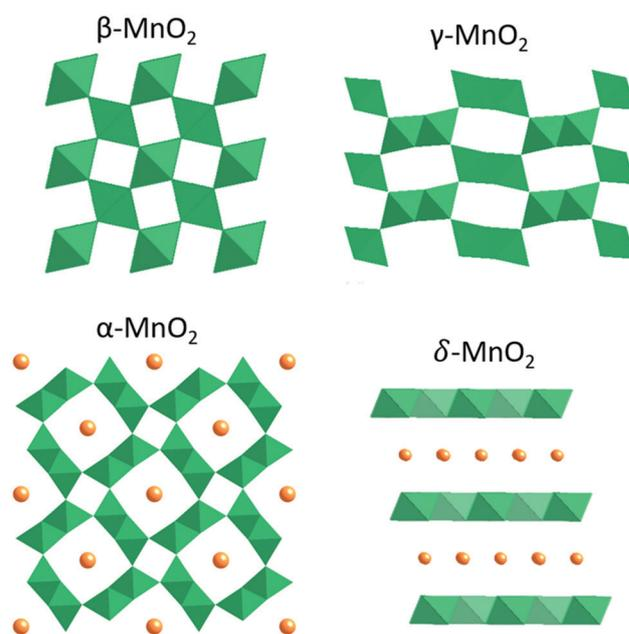
Fig. 5 Crystallographic structures of α-, β-, γ- and δ-MnO<sub>2</sub>, showing the structural cavities built from MnO<sub>6</sub> octahedra.
