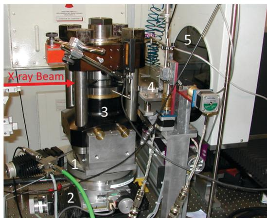
**Fig. 25** Large volume Paris–Edinburgh press on the ID27 beamline of ESRF for *in situ* angular X-ray diffraction experiments: (1) Rotation motor. (2) Micrometric motors *x*, *y* and *z*. (3) Paris–Edinburgh press. (4) Soller slits. (5) CCD detector.
