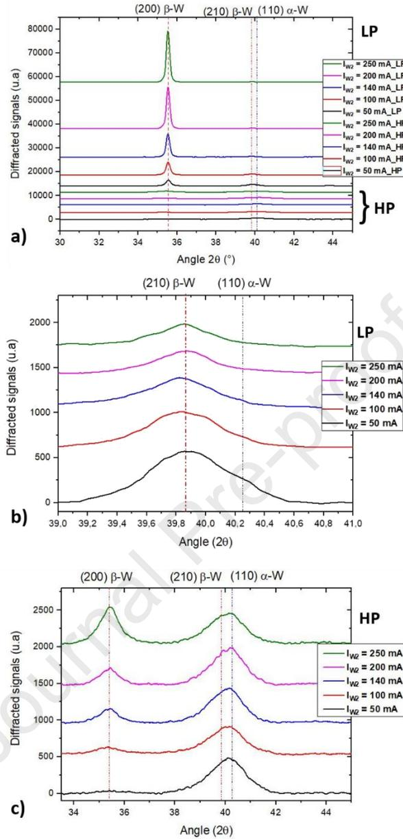
Fig. 4: X-ray diffraction patterns recorded in  $\theta/\theta$  configuration of W thin films prepared at low (LP) and high (HP) pressures with different  $I_{W_2}$  target currents: a) between  $30^\circ$  and  $45^\circ$ , b) zoom of the peak attributed to  $\alpha$ -W (110) and  $\beta$ -W (210) superposition at around  $40^\circ$  (samples deposited at low pressure) and c) between  $30^\circ$  and  $45^\circ$  (increased y-scaling) for samples deposited at high pressure.
