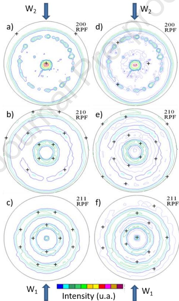
Fig. 5: a, d)  $\{200\}$ , b, e)  $\{210\}$  and c, f)  $\{211\}$  X-ray reconstructed pole figures (RPF) for the W thin films deposited at low pressure with  $IW_2 = 200$  mA. The direction of the incident fluxes, indicated by arrows corresponds to the rolling direction. The crosses correspond to theoretical texture of  $\{100\} \langle 011 \rangle$  (a-c) and  $\{211\} \langle 0-11 \rangle$  (d-f).
