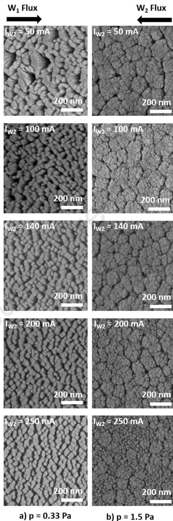
Fig. 2: Top-view scanning electron microscopy observations of W thin films deposited at a) low pressure and b) high pressure with a constant target current ( $IW_1 = 140$  mA) and various  $IW_2$  target currents.
