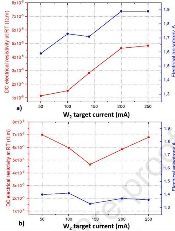
Fig. 7: DC electrical resistivity and resistivity anisotropy measured at room temperature as a function of the  $I_{W_2}$  target current for W thin films prepared by OAD with two W targets ( $I_{W_1} = 140$  mA) at a) low ( $p = 0.33$  Pa) pressure and b) high ( $p = 1.5$  Pa) pressure.
