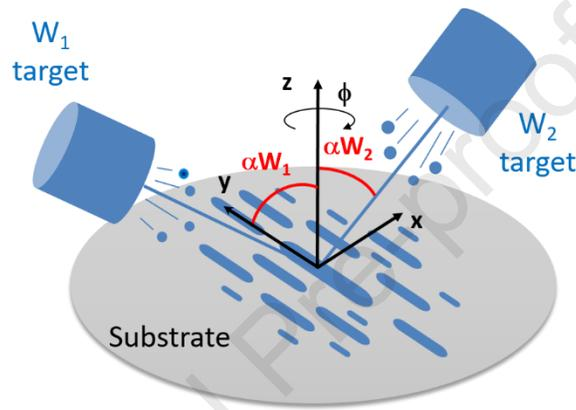
Fig. 1: Schematic representation of the OAD setup. Two tungsten targets  $W_1$  and  $W_2$  are tilted with fixed angles  $\alpha W_1 = \alpha W_2 = 80^\circ$ . The target-to-substrate distances are fixed to 65 mm for  $W_1$  and to 95 mm for  $W_2$ . The substrate can be fixed or rotated following the  $\phi$  angle (not used in this study). W atoms are deposited on substrate defining a x-y plane whereas the z-axis is defined by the direction perpendicular to the substrate.
