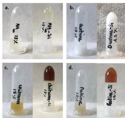
Figure 3. Gelation of Si-HA (a), Si-dextrin (b), Si-chitosan (c), and Si-pectin (d). Within each panel, the tube on the left contains non-silylated polysaccharide as control at the same concentration (13% weight).
