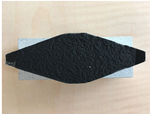
Figure 15: Example of a face of rupture ( \gamma = 0^\circ , 23^\circ\text{C} ). The marks of the pre-cracks on the left and right sides of the sample can be clearly distinguished.
