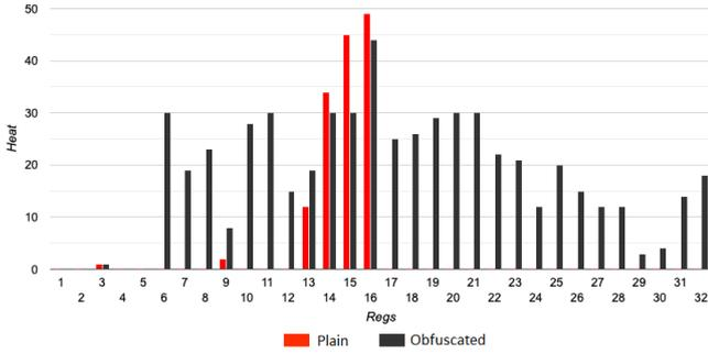
Figure 8: Register per register average  $H_r$  for SHA
