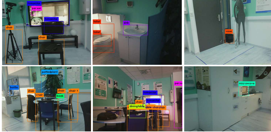
Fig. 7. 2D Object detection using YOLO-v3. The images show the detection results in different areas in the smart home.
