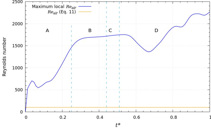
Figure 11: Evolution of the maximum local Reynolds number  $Re_{air}$  over compression time, calculated based on  $U_{z,max}$  and corresponding air thermophysical properties (Constant  $Re_{air}$  (Eq. 11) also introduced for comparison)
