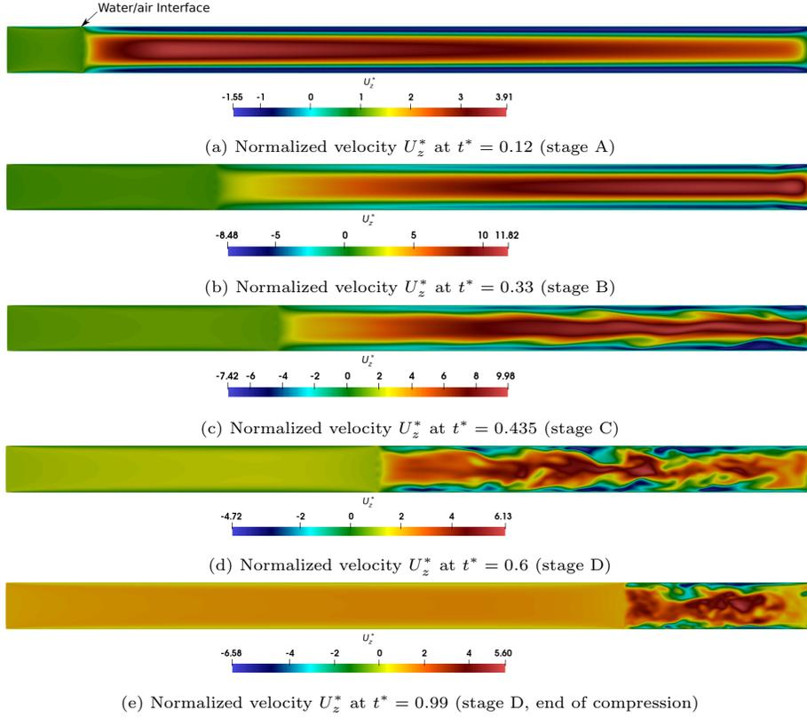
Figure 9: Velocity field  $U_z^*$  at different compression times
