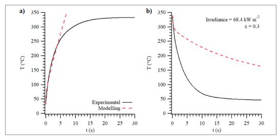
Figure 2: Measured (black full lines) and modelled (red dashed lines) surface temperature rises during laser irradiation at a 68.4 kW m-2 irradiance (2a) and falls from maximum temperature reached during irradiation (2b) of a 317 µm thick plattnerite pellet.
