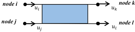
Fig. 4. Nodal boundary conditions in 1D bar kinematics.
