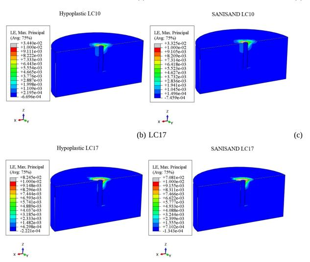
Figure 10: Distribution of the maximal principal logarithmic strain in the hypoplastic and SANISAND 3D soil domains at the end of the 10 min dynamic simulations for (a) LC10, (b) LC17
