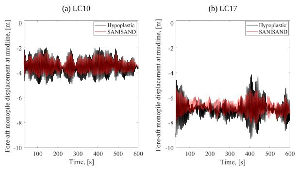
Figure 11: Fore-aft monopile displacement at mudline in [cm] as obtained by two constitutive models for (a) LC10 and (b) LC17
