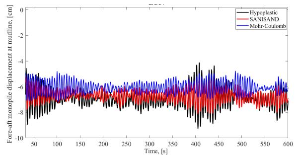
Figure 14: Comparison of the fore-aft monopile displacement at mulline in [cm] as obtained by the three soil constitutive models LC17
