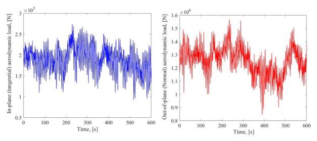
Figure 4: Tangential and normal aerodynamic loads on blade 1 for LC10.
