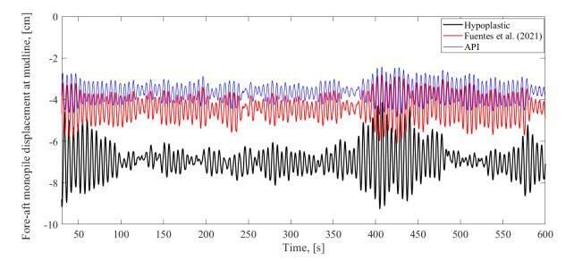
Figure 22: Fore-aft monopile displacement at mulline as obtained by the present 3D model based on hypoplasticity and the two simplified foundation models for LC17
