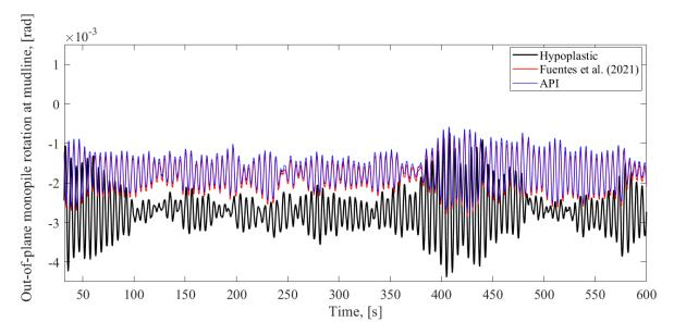
Figure 23: Out-of-plane monopile rotation time history at mudline as obtained by the present model based on hypoplasticity and the two simplified foundation models for LC17
