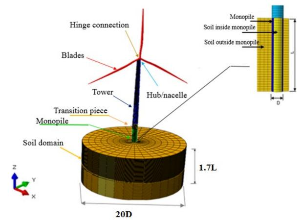
Figure 1: DTU 10 MW offshore wind turbine.
