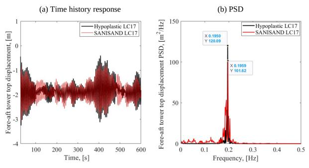
Figure 6: Fore-aft tower top displacement as obtained by two constitutive models under LC17 (a) time history and (b) frequency response spectrum
