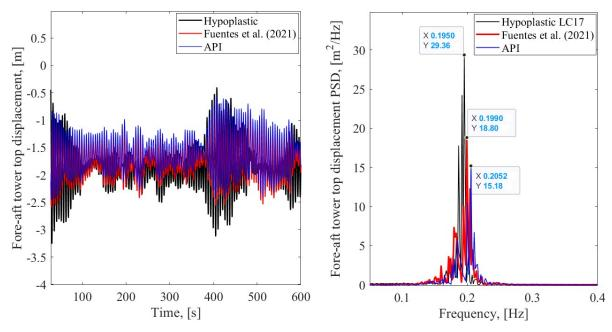
Figure 21: Fore-aft tower top displacement as obtained by the present 3D model based on hypoplasticity and the two simplified foundation models under LC17 (a) time history and (b) frequency response spectrum
