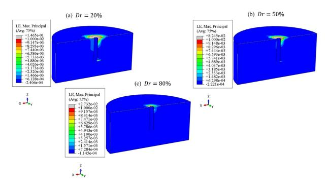
Figure 16: Distribution of the maximal principal logarithmic strain in the hypoplastic 3D soil domain at the end of the 10 min dynamic simulations for a relative density of (a) 20%, (b) 50% and (c) 80%
