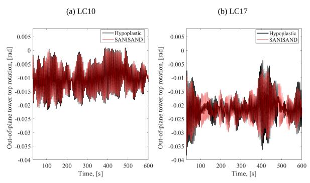
Figure 9: Tower top rotation time history as obtained by two constitutive models for (a) LC10 and (b) LC17
