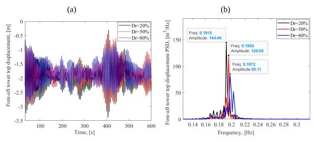
Figure 15: Fore-aft tower top displacement as obtained using the hypoplastic constitutive model for three sand relative densities (20%, 50% and 80%) (a) time histories and (b) frequency response spectrums
