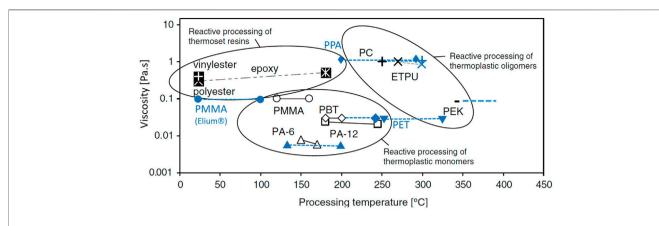
FIGURE 1 | Processing temperature and viscosity ranges of various polymers suitable for reactive processing (adapted from (van Rijswijk and Bersee, 2007), plotted in black and white, and (Qin et al., 2020), plotted in blue).
