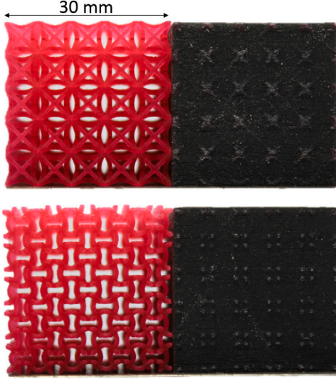
Fig. 2. Lattice samples of Hexaround and Warmuth structures after manufacturing (left side) shown in red and their composite counterparts filled with TangoBlack+ hyperelastic materials (right side).
