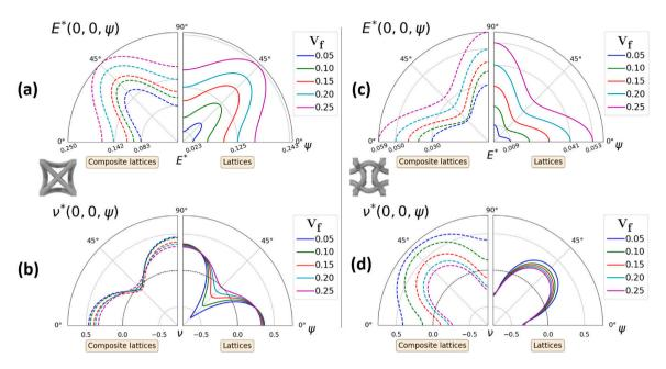
Fig. 6. Hexaround (left) and Warmuth (right) elastic properties depending on loading orientation and lattice volume fraction.
