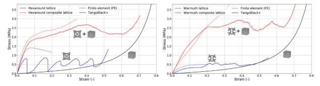
Fig. 10. Strain/stress plot, Hexaround (left) and Warmuth (right).
