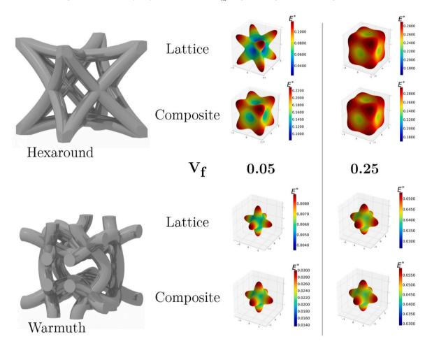
Fig. B.14. 3D representation of the normalized directional elastic stiffness (Young's modulus as a function of orientation) for Hexaround and Warmuth cells at 0.05 and 0.25 volume fraction for both truss and composite lattices.
