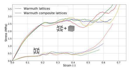
Fig. C.16. Sress/strain plot, Warmuth lattices and composite lattices compression test.
