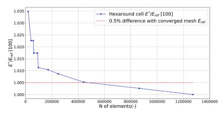
Fig. A.12. Mesh sensitivity study for the Hexaround cell.  $E_{\rm ref}$  being the converged normalized Young's modulus.
