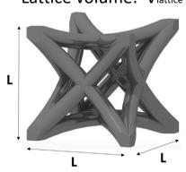
Fig. 5. Representation of  $V_{\text{cubic}}$  and  $V_{\text{lattice}}$ .
