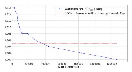
Fig. A.13. Mesh sensitivity study for the Warmuth cell.  $E_{\rm ref}$  being the converged normalized Young's modulus.
