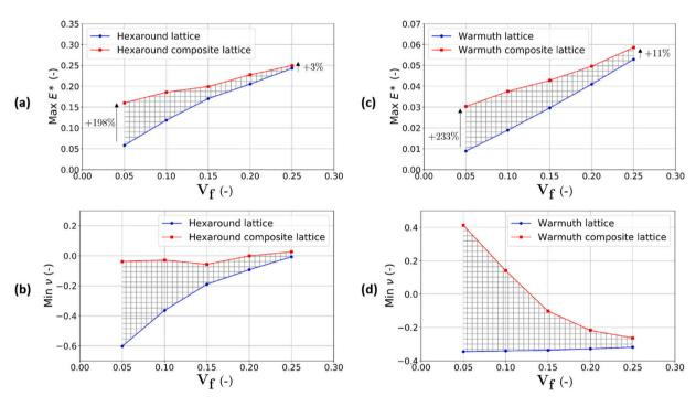
Fig. 7. Influence of the filling soft phase on maximum normalized modulus (a)(c) and minimal Poisson's ratio (b)(d), for different lattice volume fraction.
