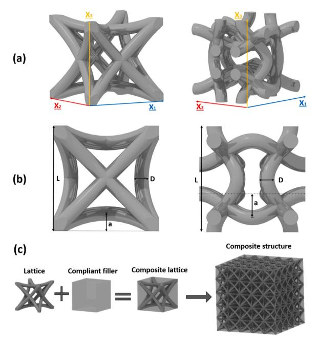
Fig. 1. Hexaround (left) and Warmuth (right) unit-cells, with their periodicity vectors  $\underline{X_i}$  (a), and geometric descriptions (b), and the strategy to create composite lattice structures (c).
