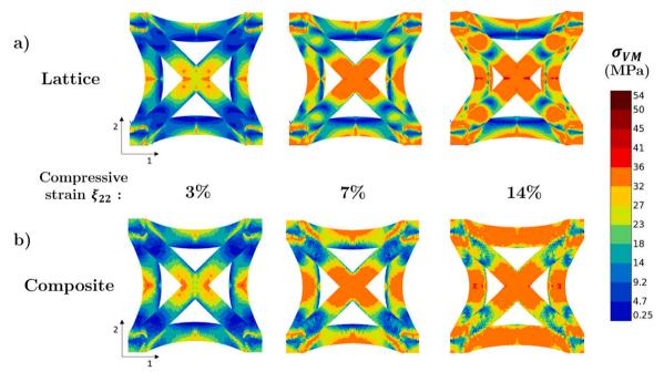
Fig. 9. Von Mises equivalent stress maps within the truss for both simple (a) and composite (b) lattices at 3 levels of uniaxial compressive strain, resulting from FE simulations.
