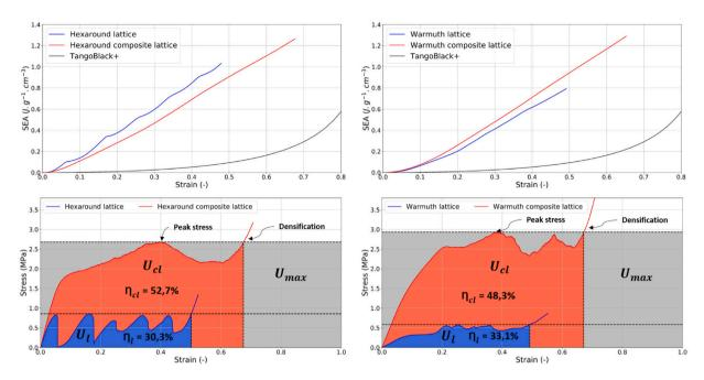
Fig. 11. SEA and Efficiency plot, Hexaround (left) and Warmuth (right).
