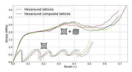
Fig. C.15. Stress/strain plot, Hexaround lattices and composite lattices compression test.
