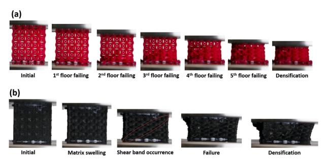
Fig. 8. Change in the mode of failure from layerwise for the hexaround lattice (a) to shear band for the composite hexaround lattice (b).
