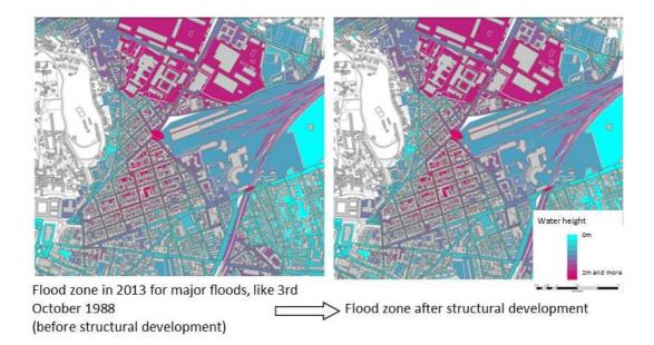
*Figure 3: evolution of the flood zones before and after structural development, for minor (above) and major (below) floods. Provided by the city of Nîmes*
