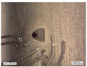
Fig. 6: Shaped Hole at  $1100^{\circ}$ C in the furnace: presence of 3 thermosensors for temperature acquisition.
