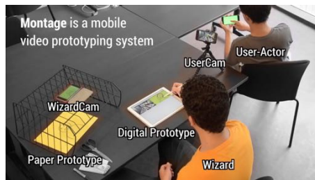
Figure 1: An overview of the MONTAGE video prototyping system. Here, two designers, a wizard and a user-actor, collaborate side-by-side. The UserCam captures the user-actor enacting user inputs in the actual context, i.e. using his phone at the office. The WizardCam captures the paper prototype and the Canvas captures the wizard's digital sketches.
