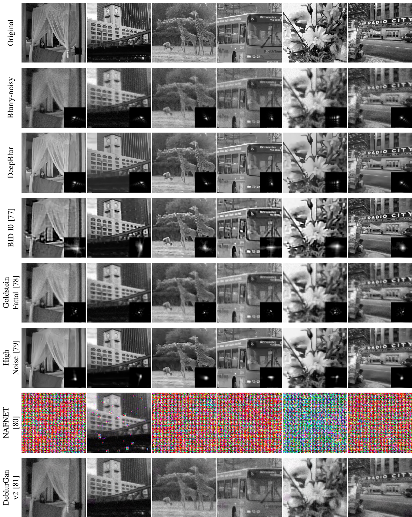
Fig. 9: Deep-Blur in action with additive white Gaussian noise and \sigma = 5 \cdot 10^{-2} . Quantitative evaluations are reported in Table II. When available, the estimated blur kernel is displayed at the bottom-right. First row : original images. Second row : blurry-noisy images. Third row : Deep-Blur. Fourth row : [77] Fifth row : [78] Sixth row : [79] Seventh row : [80] Eith row : [81]
