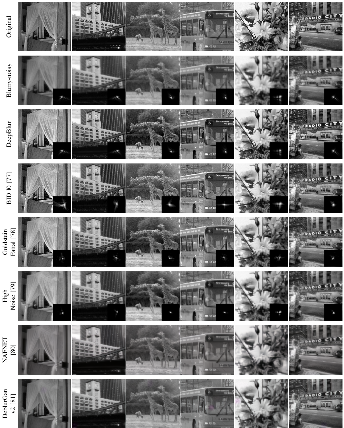
Fig. 8: Deep-Blur in action with additive white Gaussian noise and \sigma = 10^{-2} . Quantitative evaluations are reported in Table II. When available, the estimated blur kernel is displayed at the bottom-right. First row : original images. Second row : blurry-noisy images. Third row : Deep-Blur. Fourth row : [77] Fifth row : [78] Sixth row : [79] Seventh row : [80] Eith row : [81]
