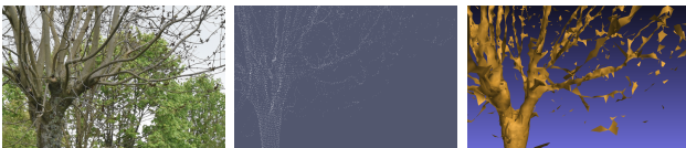
Fig. 1: Challenges with meshing: (a) the real tree, (b) the point-cloud from the Total Station (c) an example of mesh failing to describe the actual surface of the fine elements of the tree.
