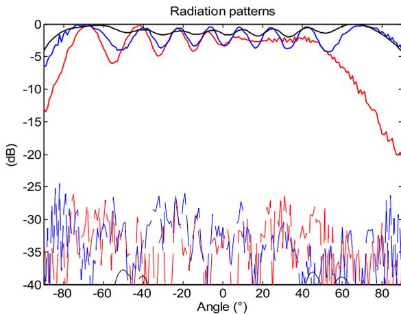
**FIGURE 11. Co-polar (red solid line) and cross-polar (red dashed line) of measured radiation pattern in E plane for antenna 1 at 76 GHz. Co-polar (blue solid line) and cross-polar (blue dashed line) of measured radiation pattern in E plane for antenna 2 at 76 GHz. Co-polar (thin solid line) and cross-polar (thin dashed line) of simulated radiation pattern in E plane for antenna 1 at 78.5 GHz.**
