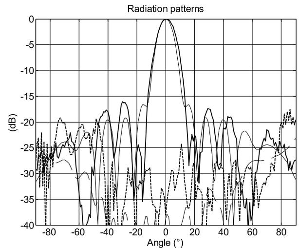
**FIGURE 10.** Co-polar (thick solid line) and cross-polar (thick dashed line) of measured radiation pattern in H plane at 76 GHz. Co-polar (thin solid line) and cross-polar (thin dashed line) of simulated radiation pattern in H plane at 78.5 GHz.
