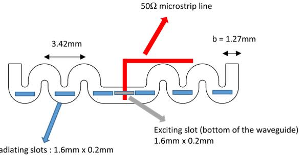
**FIGURE 12. Antenna 2: Designed serpentine waveguide with dimensions.  $b$  is the narrow width of the waveguide. Radiating slots are in blue, and the center slot is on the bottom of the waveguide to excite it from a bended 50- $\Omega$  microstrip line (antenna 2).**
