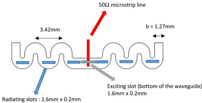
**FIGURE 8.** Antenna 1: Designed serpentine waveguide with dimensions. *b* is the narrow width of the waveguide. Radiating slots are in blue, and the center slot is on the bottom of the waveguide to excite it from the 50-Ω microstrip line.
