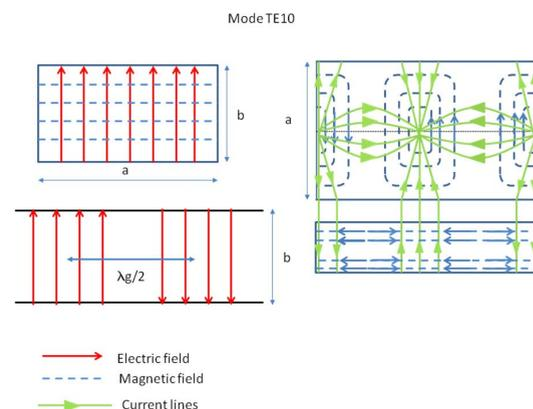
**FIGURE 1.** Electric/magnetic field distributions and current lines for the fundamental TE<sub>10</sub> mode in a rectangular waveguide ( $a$  and  $b$  are, respectively, the width of the broad and narrow walls).
