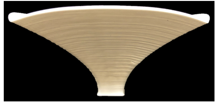
Figure 5: Manufactured square shaped tube: zero-phase moving average filtering smoothing.
