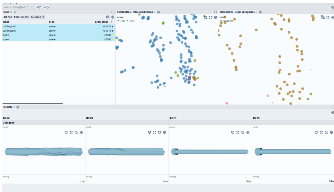
Fig.2: Prediction scores, ground truth values and embeddings are used to qualitatively understand and improve a training dataset for 3D object classification.
