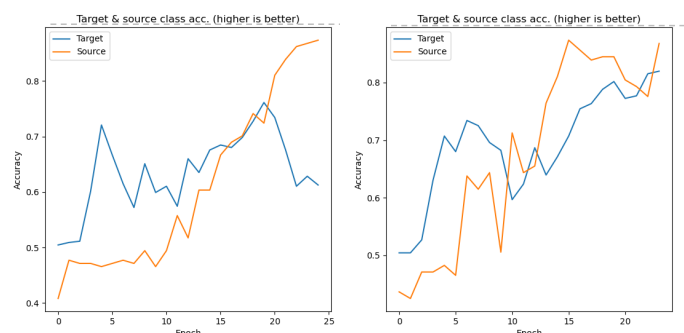
Fig. 3: Validation accuracy per epoch per domain without domain adaptation (left) vs. MuLANN (right).
